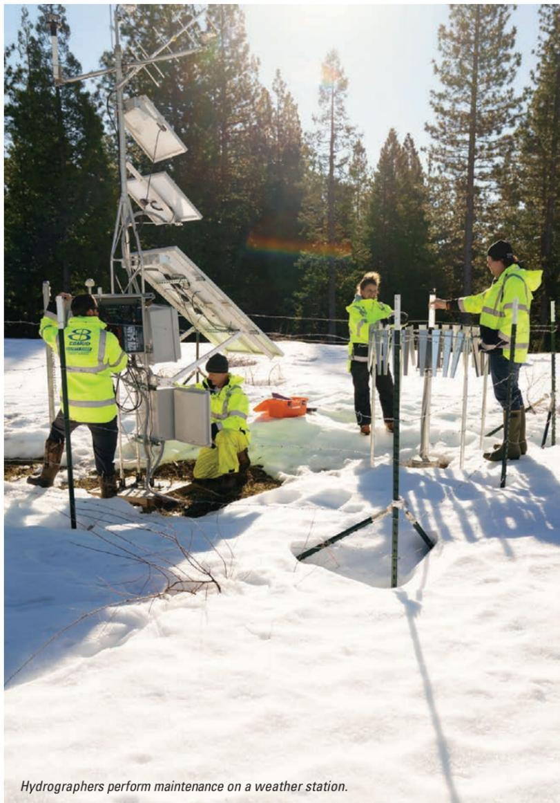
Hydrographers perform maintenance on a weather station.
