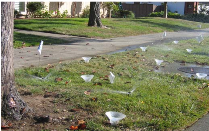
Existing sprinkler uniformity tested poorly at 48%
